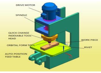
Engine is begun which turns the fundamental shaft at fast. The device or bolt set mounted in the apparatus holder pivots at rapid. The employment to be bolted alongside the bolt is set in the work holder .The encourage engine is worked to move in upward heading to lift the table slide and table in the table guide by means of roller plan.
